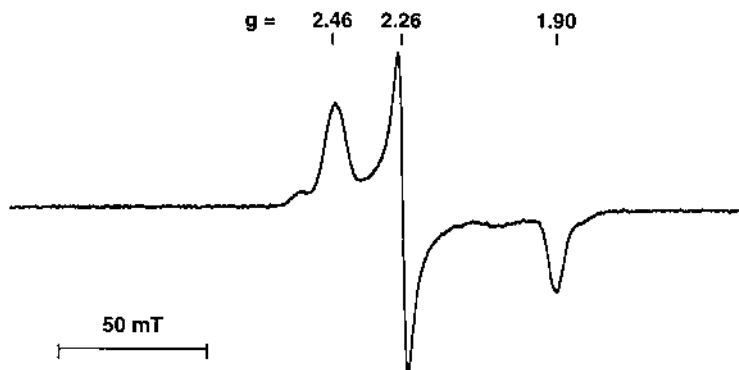
Fig. 2. X-band EPR spectra of wild-type CooA. The microwave power, modulation frequency, modulation amplitude, and measurement temperature are 1 mW, 100 kHz, 1 mT, and 77 K, respectively.
